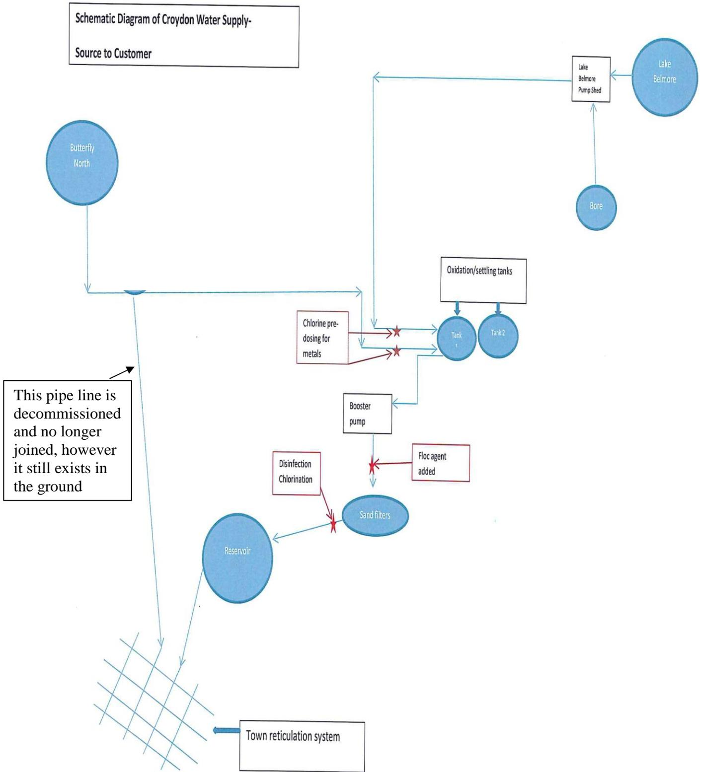
Figure 2.3 Treatment Plant Schematic
